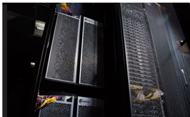
EIDF, operated by EPCC, includes Cerebras CS-3 systems configured as a Wafer-Scale Cluster. Image: Andrew Perry.
