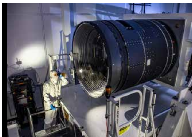
The 3200 megapixel camera that will take images for Rubin Observatory's 10-year Legacy Survey of Space and Time. (Jacqueline Ramseyer Orrell/SLAC National Accelerator Laboratory).
