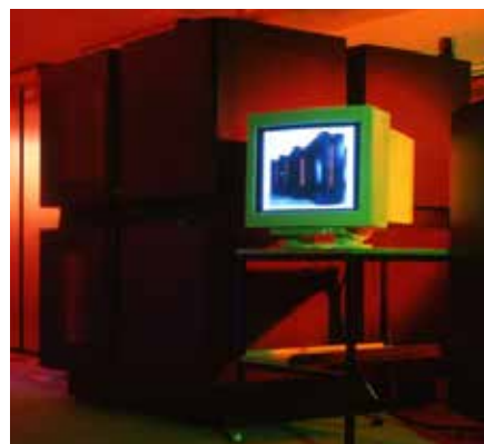
The 16,384-processor Connection Machine (CM-200) from Thinking Machines Corporation was the first system run by EPCC as a national supercomputing service for UK academia and industry.
