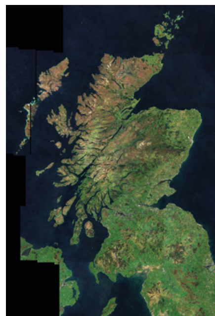
Multispectral cloud-free composite image (showing combined RGB channels) produced by combining Sentinel-2 images from Summer 2019 produced using Data Slipstream by the School of Geosciences and EPCC staff on the EIDF.
