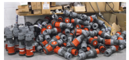
Above: Some of the removed 125 amp 3-Phase plugs.
